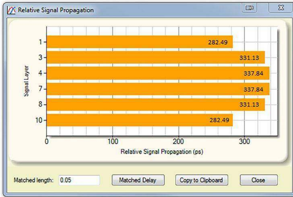
Figure 5: Relative signal propagation of microstrip and stripline, simulated in iCD Design Integrity.
