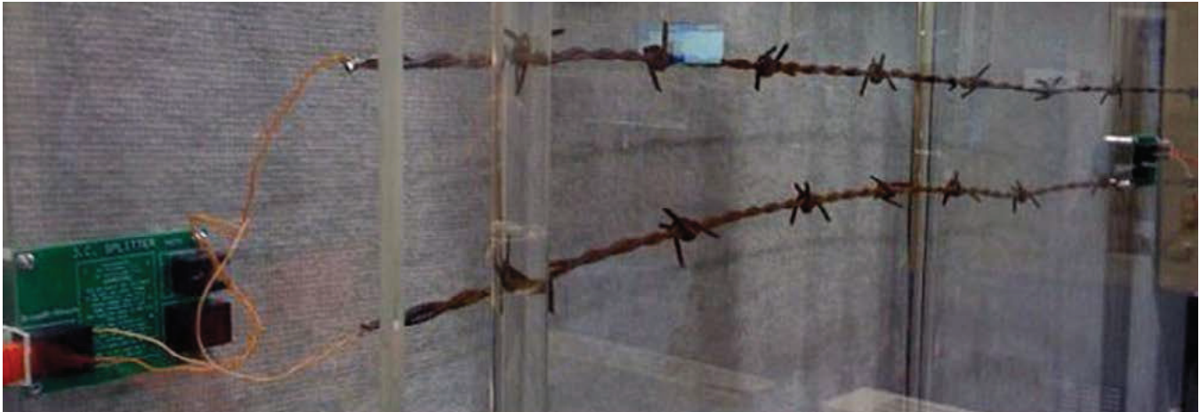
Figure 2: Broadcom Fast Ethernet 100Base-T4 over barbed wire (courtesy Broadcom).
