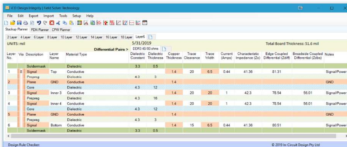
Figure 5–A six layer stackup top/bottom microstrip and middle dual stripline (ICD Stackup Planner)
