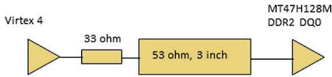
Figure 2: DDR2 data signal with series terminator.
