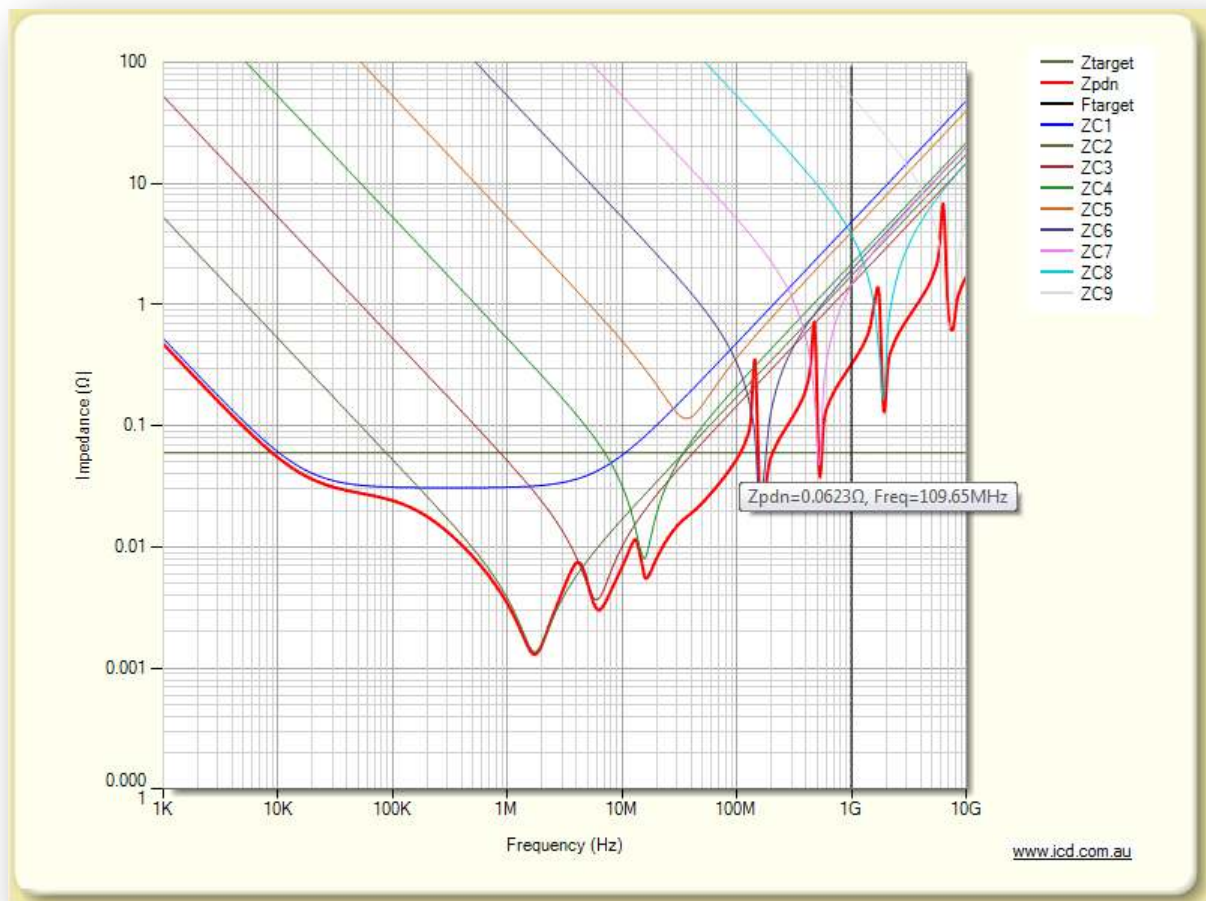
Figure 4 – One value capacitor per decade approach
