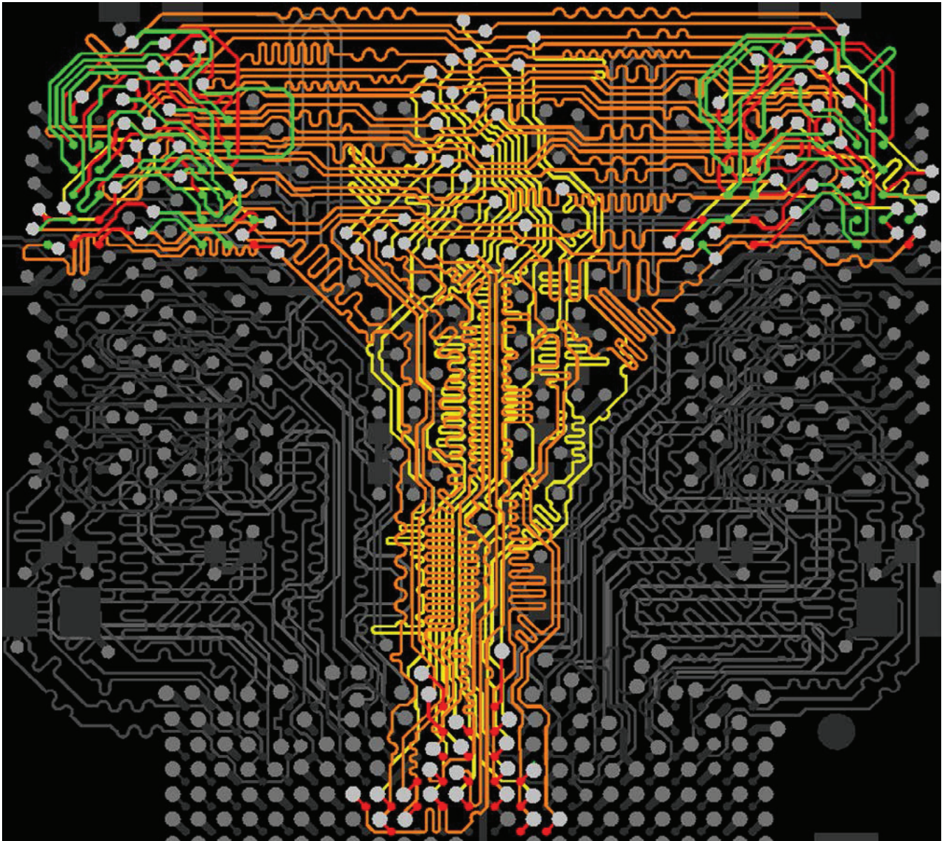
Figure 1: Matched delay T-section DDR2 address routing in Altium Designer.
