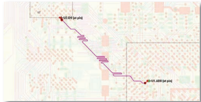
Figure 8. DQ5 routed on inner layer 3.
