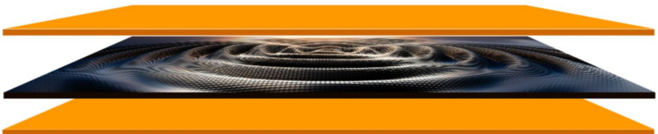
Figure 1: A standing wave built up by plane cavity resonance.
