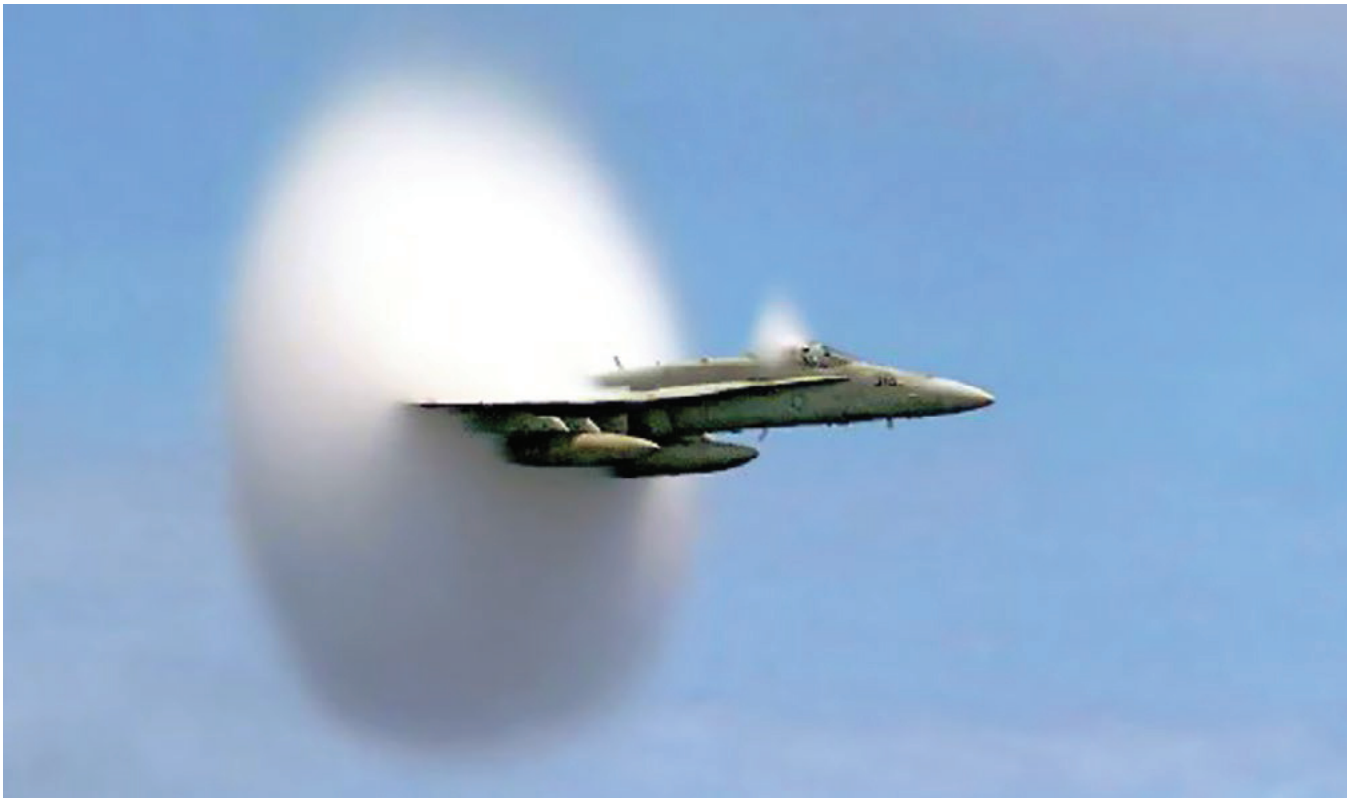
Figure 1: An FA-18 approaches the speed of sound. The white halo consists of condensed water droplets formed by the sudden drop in air pressure behind the shock cone around the aircraft. (Courtesy of the U.S. Navy)
