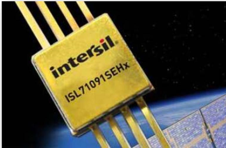
Figure 3 – RAD HARD device (courtesy Intersil)
