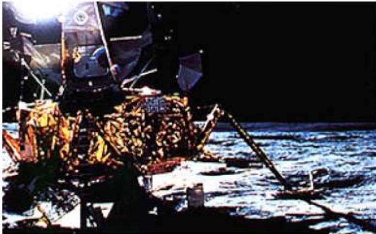
Figure 2 – Gold foil acts as a radiation shield on the Apollo lunar module
