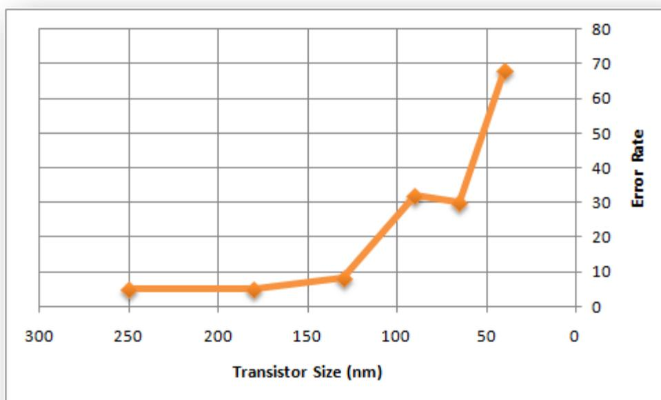
Figure 1 – Transistor size vs microprocessor error rate (source Oracle)
