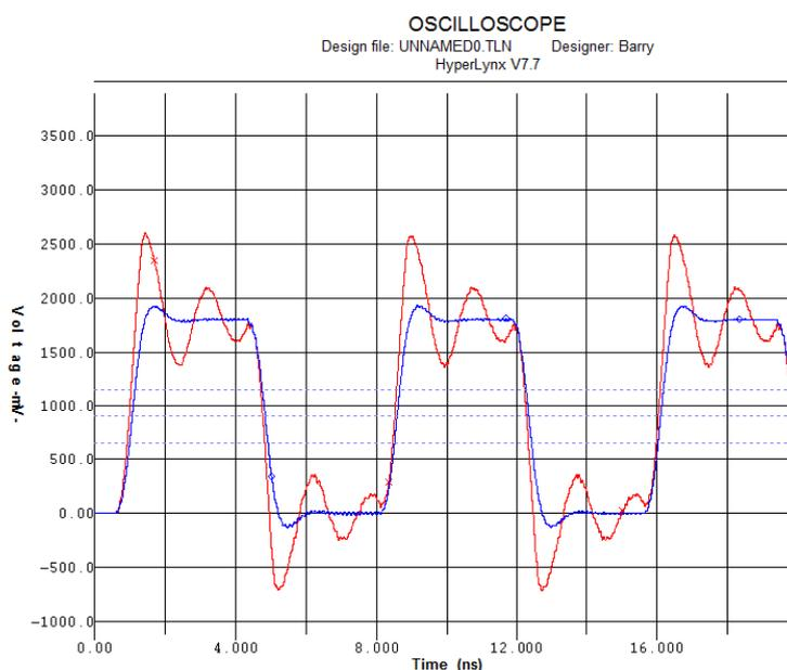
Figure 1 – Unterminated (red) vs terminated (blue) transmission lines
