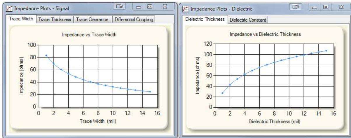
Figure 2 – the ICD Stackup Planner’s impedance plots
