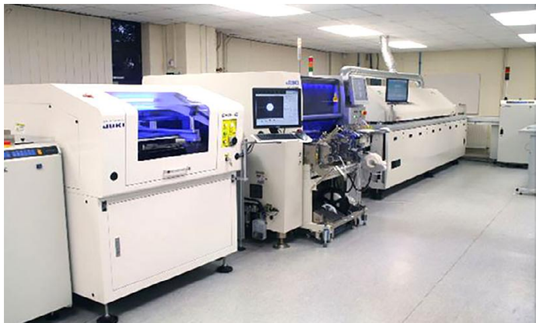
Figure 2: SMT assembly production line (Courtesy Juki).
